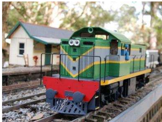
Primer coat, next mask for yellow stripes, then Green paint, ready to blacken handrails.
