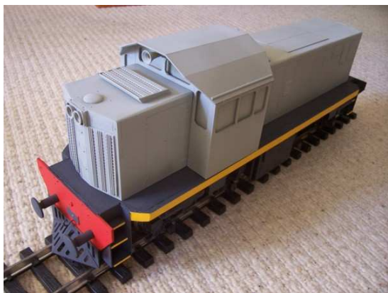
Primer coat, next mask for yellow stripes, then Green paint, ready to blacken handrails.
