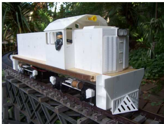
Cab sides drilled and cut outs for windows. Cab, short & long HOODS assembled. The QR style Cow Catcher mounted on the Buffer Plate ready for Buffers and Coupler.
