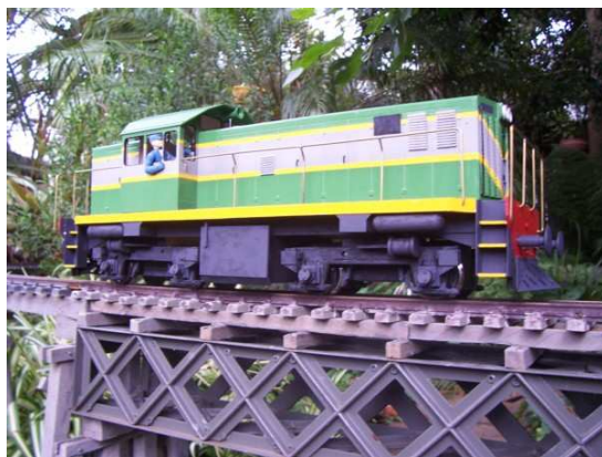
Primer coat, next mask for yellow stripes, then Green paint, ready to blacken handrails.
